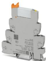
PLC-INTERFACE, consisting of basic terminal block PLC-BSC.../21 with screw connection and plug-in miniature relay with power contact, for assembly on DIN rail NS 35/7,5, 1 changeover contact, input voltage 24 V DC
