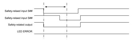
Both safety-related inputs are deactivated within the signal interlock monitoring time of 200 ms. When they are activated again, the safety-related outputs are also activated.
